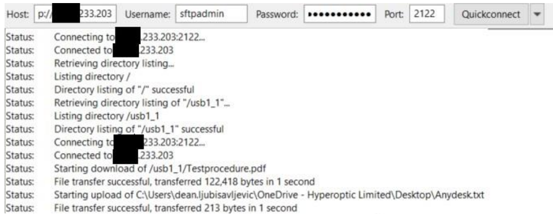
Image 21. Access to USB flash drive via FileZilla client app (from WAN)
